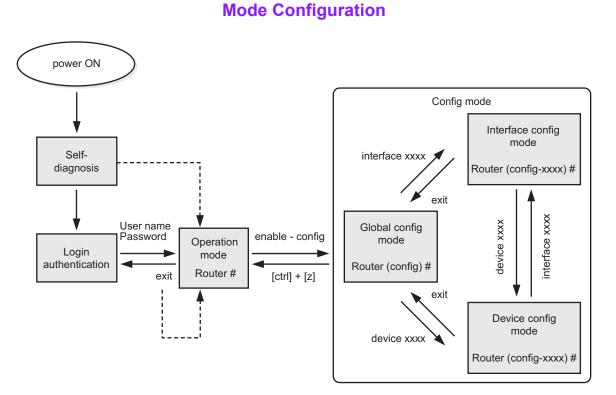
The characters "Router" preceding the prompt on the screen is the default setting. If you set a host name using the hostname command for router identification purposes, "Router" is replaced by this host name.
